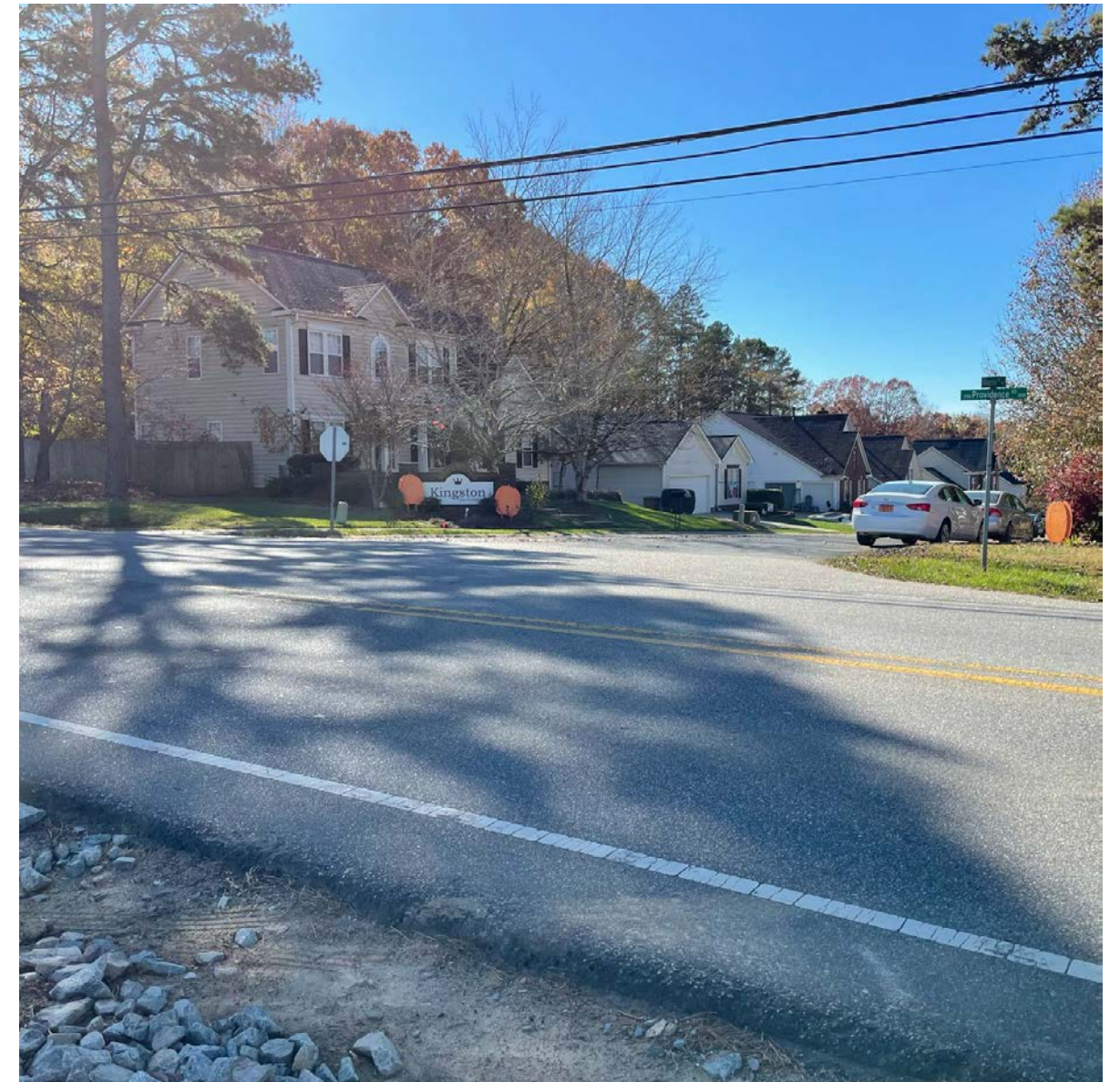
Person-level view of existing two-lane roadway and lack of controlled crossing at Kingston Dr at NC-16. The roadway is planned for widening in 2027 to a multi-lane roadway with sidewalk on the westside and SUP on the east side. Credit: Town of Waxhaw
