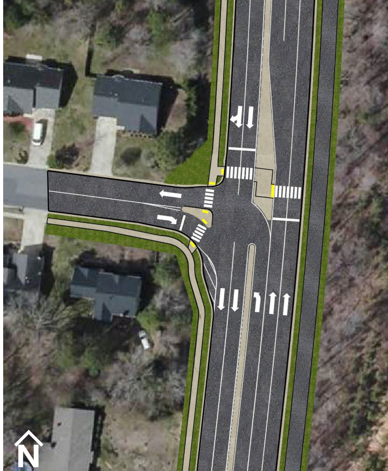
Aerial conceptual rendering of Project Int-43, showing the proposed controlled pedestrian crossing at the Kingston Dr intersection that would provide access to the SUP on the east side of the road as part of TIP U-5769A.
