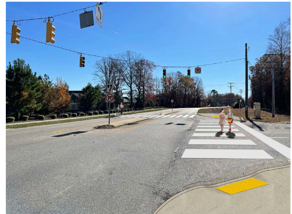
Project Int-06 conceptual rendering from person-level perspective showing the improved intersection with pedestrian phase and marked crosswalks.
