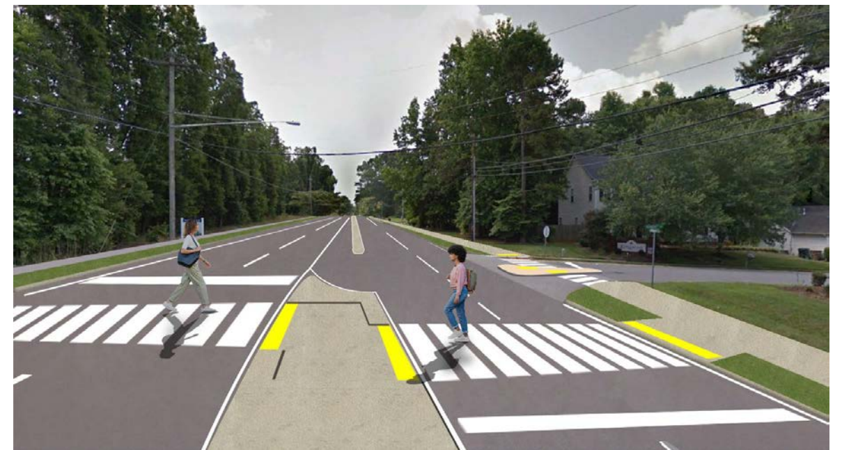
Project Int-43 conceptual rendering from person-level perspective showing the inclusion of the controlled pedestrian crossing at the Kingston Dr intersection that includes high visibility marked crosswalks and a pedestrian refuge island.
